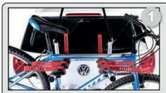
If the frame triangle fits over the tubes, simply hang the bicycle on the two top corners. Mount the bicycle(s) as close as possible to the car.
