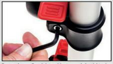
Ensure the cradles sit in position securely by tightening the screw at the bottom.
