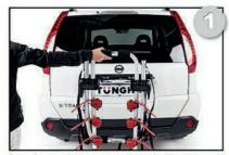
Start fitment by orienting the rack. The adjusters above, 'elbows' below, pointing away from vehicle.
