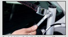
Regularly tighten the buckle bolt (with a no. 10 spanner) to ensure the buckles remain secure.
