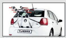
Rack to be positioned in the centre. Re-tighten all the belts once the rack has been mounted.
