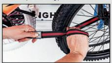
Weave the securing belt through the wheels to minimise twisting and turning during transit.
