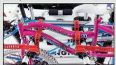
If the frame triangle doesn't fit over the tubes, mount the one cradle inside the triangle and the other below (outside) the triangle.
